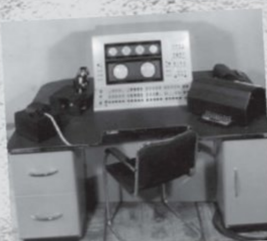
THE MARK I'S OPERATOR CONSOLE. SHOWING ITS CRT BASED MEMORY BANKS.
