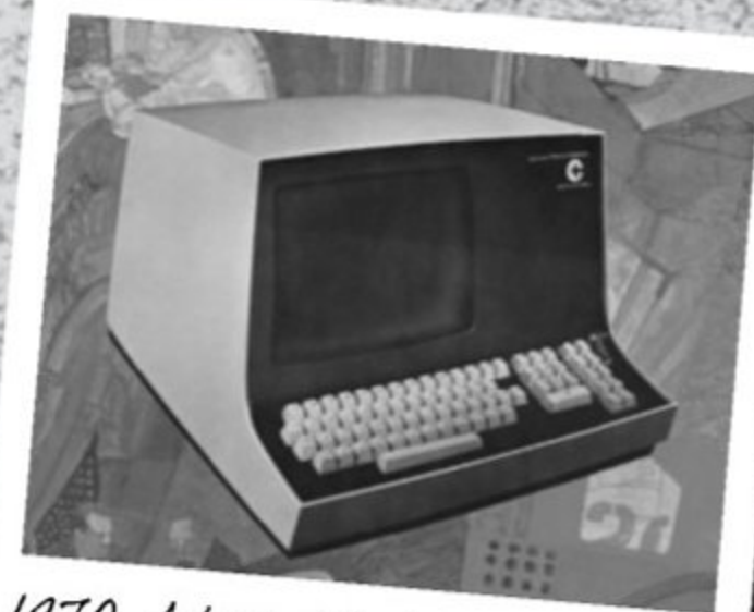
1970 A typical text-data terminal that came in to wider use during the late Sixties. Many of the text-based games written in BASIC or FOCAL would have been programmed and played on terminals like this.
